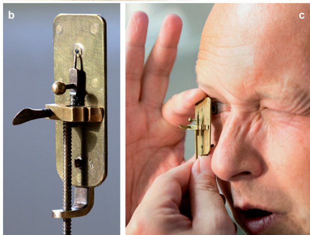
Fig. 1a-c: Antonie van LEEUWENHOEK and his type of microscope. a – The portrait shows Antonie van LEEUWENHOEK at the age of 54 years (etching by Jan VERKOLJE [1650–1693], Rijksmuseum Amsterdam, 1686). b – The single-lens microscope. c – Handling of the LEEUWENHOEK-microscope.
