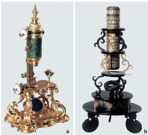
Fig. 13a, b: Splendour microscopes. a – A baroque device after Duc de CHAULNES, around 1760. b – A Japanese instrument of the 19th century.
