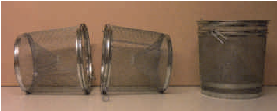
Fig. 8: Minnow traps can be taken apart into two pieces for a space-saving transport: Minnow trap type “Gee 48” taken apart into two pieces (left) and fitted into each other (right). Photo: A. Kronshage.
