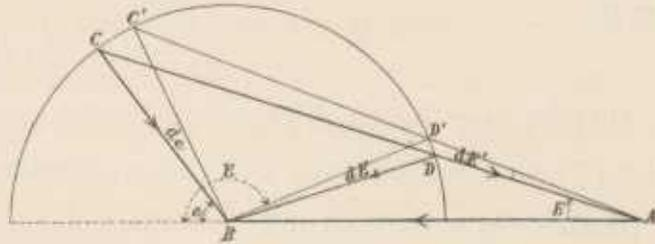
$$\left. \begin{aligned} CA = v &= n \cos E' + \sqrt{c^2 - n^2 \sin^2 E'} \\ DA = v' &= n \cos E' - \sqrt{c^2 - n^2 \sin^2 E'} \end{aligned} \right\} 4) a.$$
