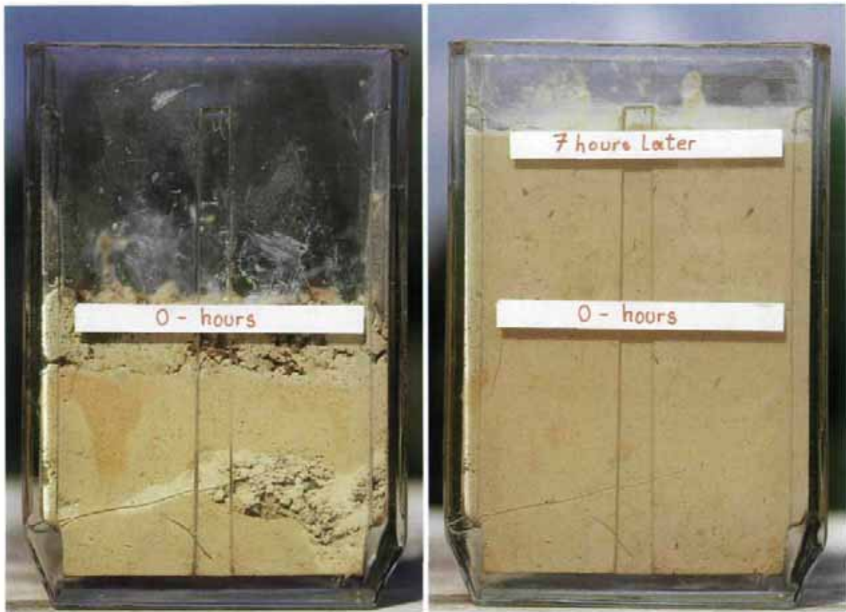
Fig. 250, 251. Sampling site (57): The Pan soil is a mixture of clay, lime, and salt, pH 7.6–9.7. The air-dried mixture (Fig. 250) is like a stone, but quickly doubles its volume and becomes a fluffy pancake when rewetted (Fig. 251).
