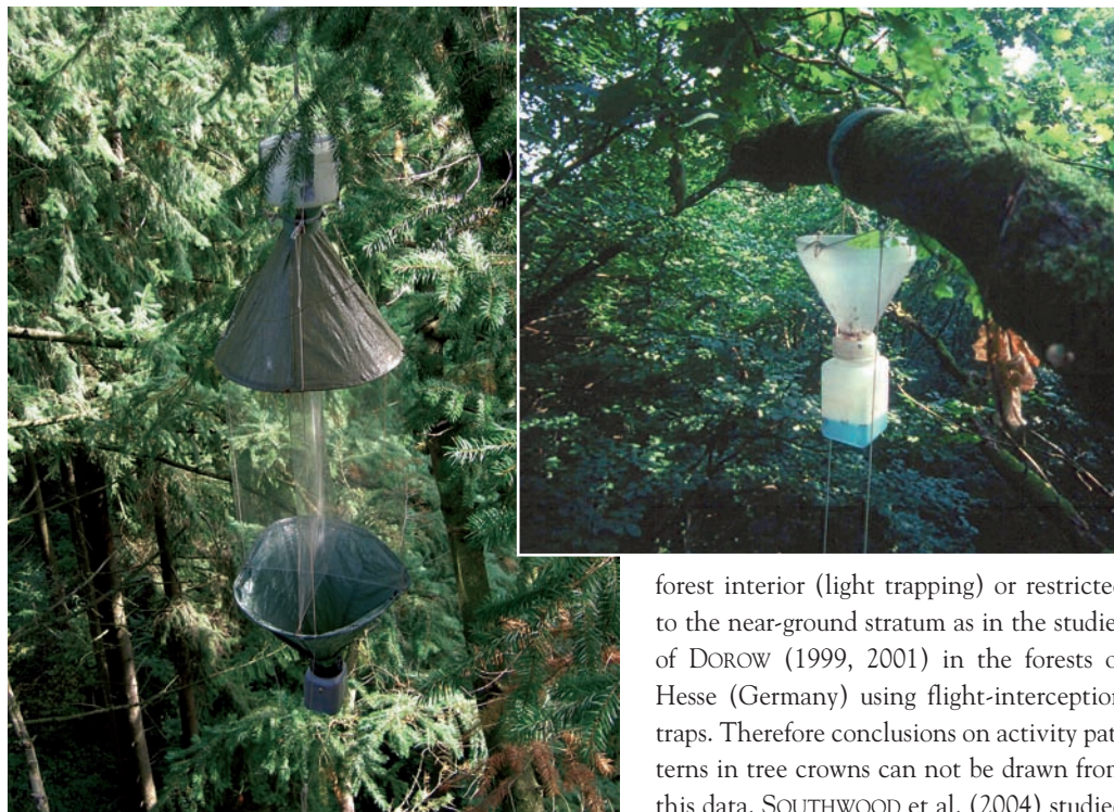
Fig. 1: a) Flight-interception trap in the canopy of Pseudotsuga menziesii and b) branch-trap in the canopy of Quercus robur .
