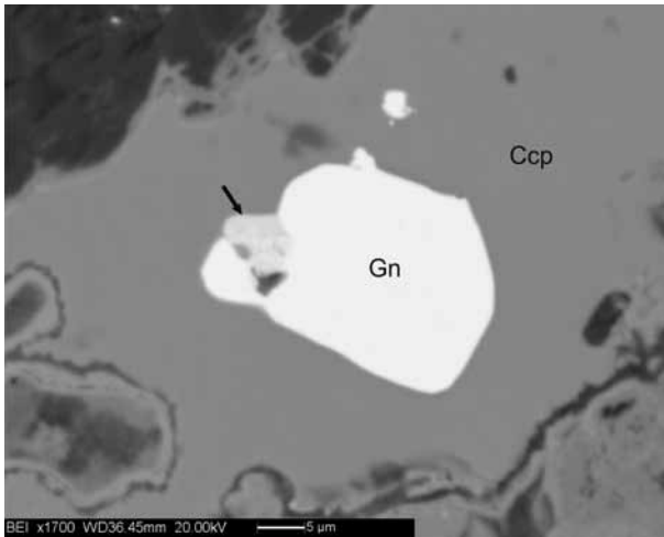
Fig. 26. Chalcopyrite (Ccp) enclosing galena (Gn) with strongly argentiferous Bi sulfosalt (arrow).
