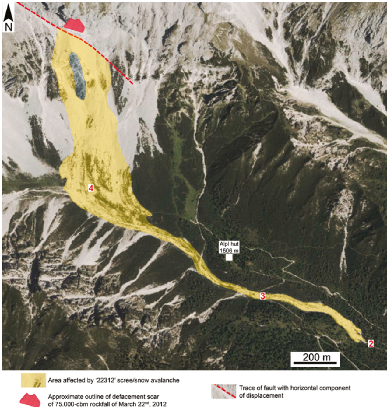
Fig. 3: Satellite orthoimage showing depositional area of the 22312-scree/snow avalanche.
