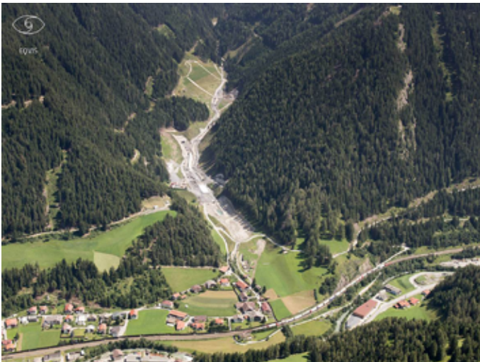
Fig. 6: Overview of the Padaster valley. a) Current view of the Padaster valley and of the village of Siegreith: The construction (bulk tunnel, diversion tunnel) is completed; the depositing of excavated material is in progress. b) After the depositing of excavated material is completed the Padaster valley will be fully recultivated (reforestation, new stream course, ecological compensation areas, etc.).
