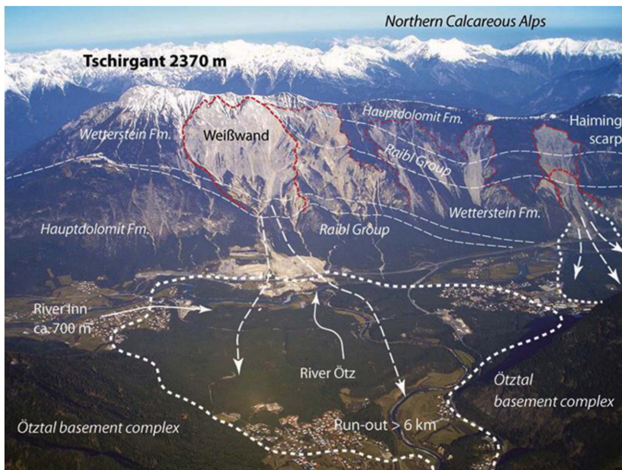
Fig. 8: Oblique view from the northern Ötz valley to the Inn-valley and Tschirgant massif. Scarp (red stippled) and accumulation areas (white stippled) of the Tschirgant and Haiming rock avalanches. The major tectono-stratigraphic units are indicated schematically, complex fold and fault structures here not depicted (from Prager et al., 2008).
