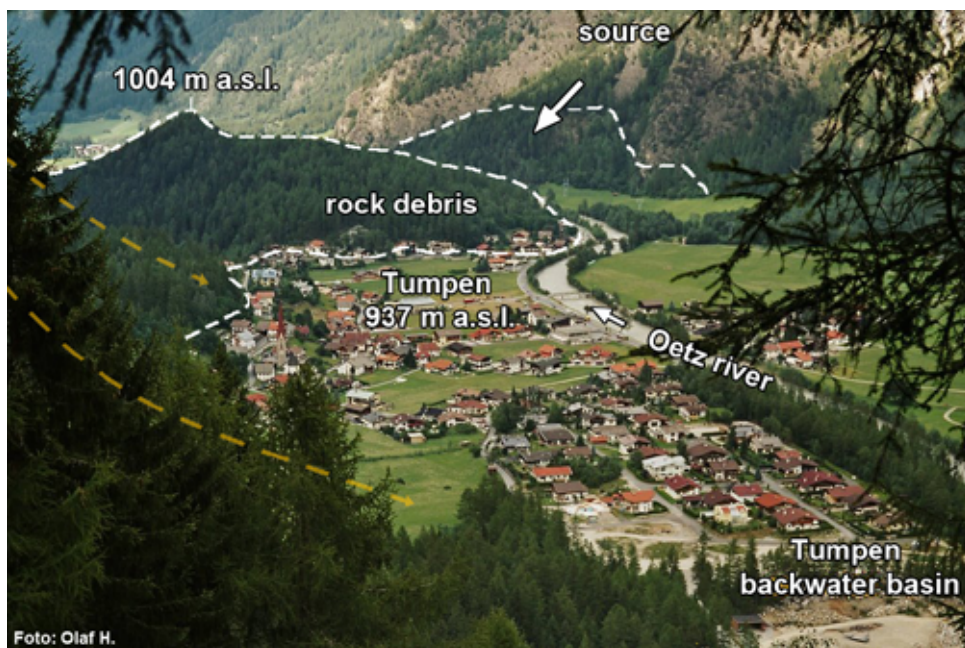
Fig. 13: Oblique view of the Oetz valley at Tumpen towards North. The valley was dammed by the Tumpen/Achplatte rock avalanche and the Tumpen backwater basin filled up with fluvio-lacustrine sediments. Other landslide events in the area Tumpen village (Poscher & Patzelt, 2000) here only indicated schematically (orange lines). The river Ötz incised into the rock avalanche debris (granodiorite gneiss) and now cascades down over a vertical distance of 90 m within just about 500 m in horizontal distance, known as the “Achstürze”.
