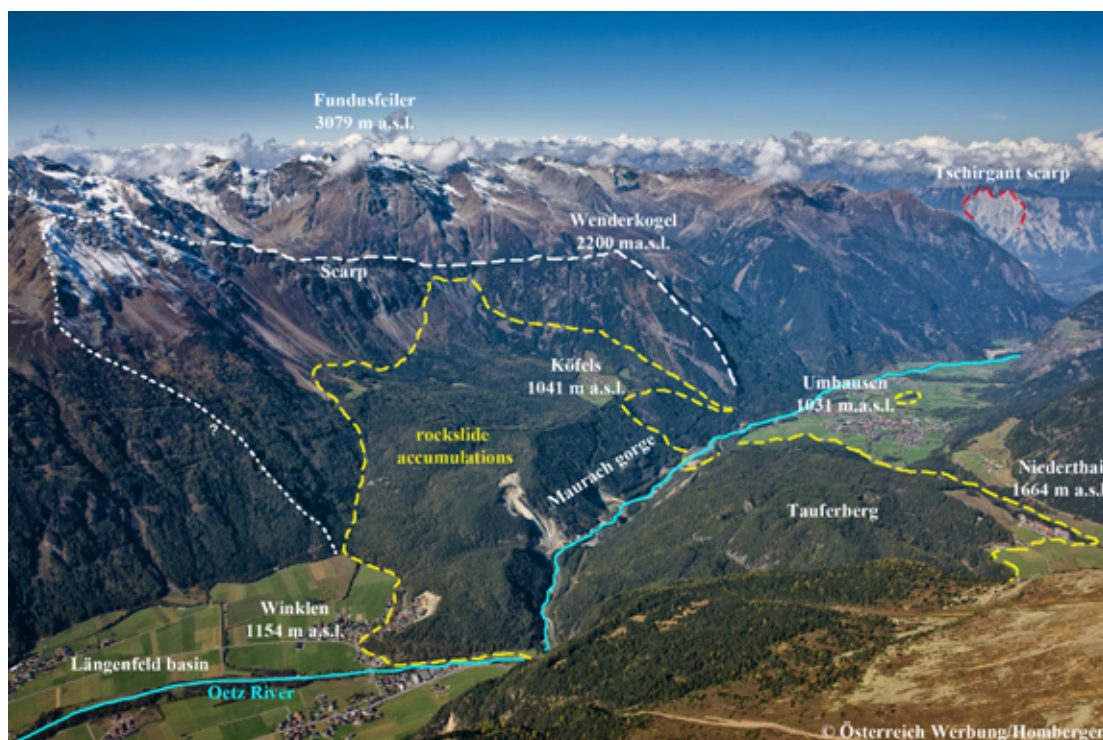
Fig. 15: Overview image of the Köfels rockslide area view towards WNW. The rockslide mass detached along East-dipping sliding planes and fully dammed the Ötztal valley. The resulting Längenfeld backwater basin was filled up with decametre-thick fluvio-lacustrine sediments. Now the river Ötztal is deeply incised in the rockslide debris, forming the Maurach gorge but not exposing the base of the rockslide yet.
