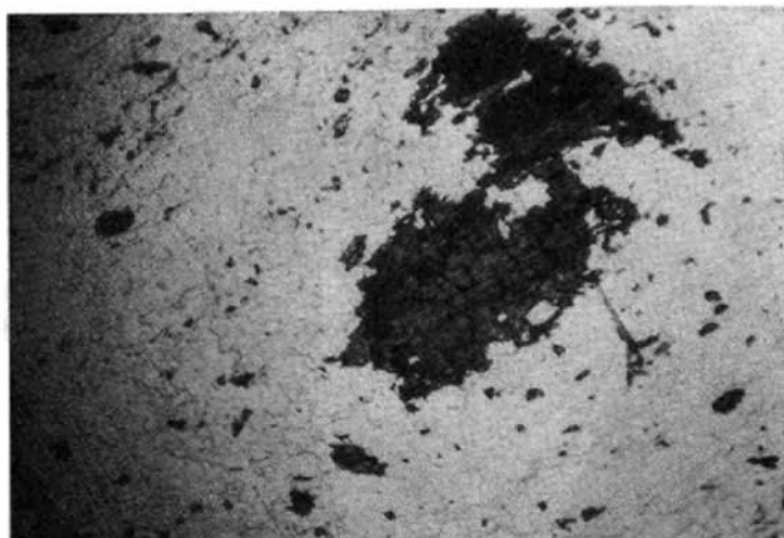
Photo 2. Primary riebeckite in riebeckite gneiss ( \times 35 ).
