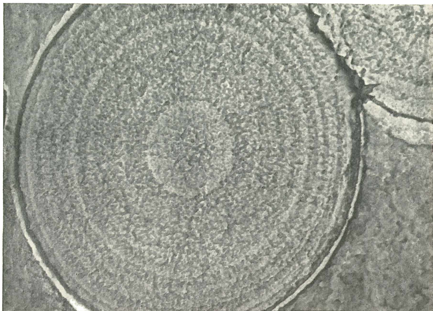
Fig. 17 Particles of carbonyl iron powder. 15.000:1.
