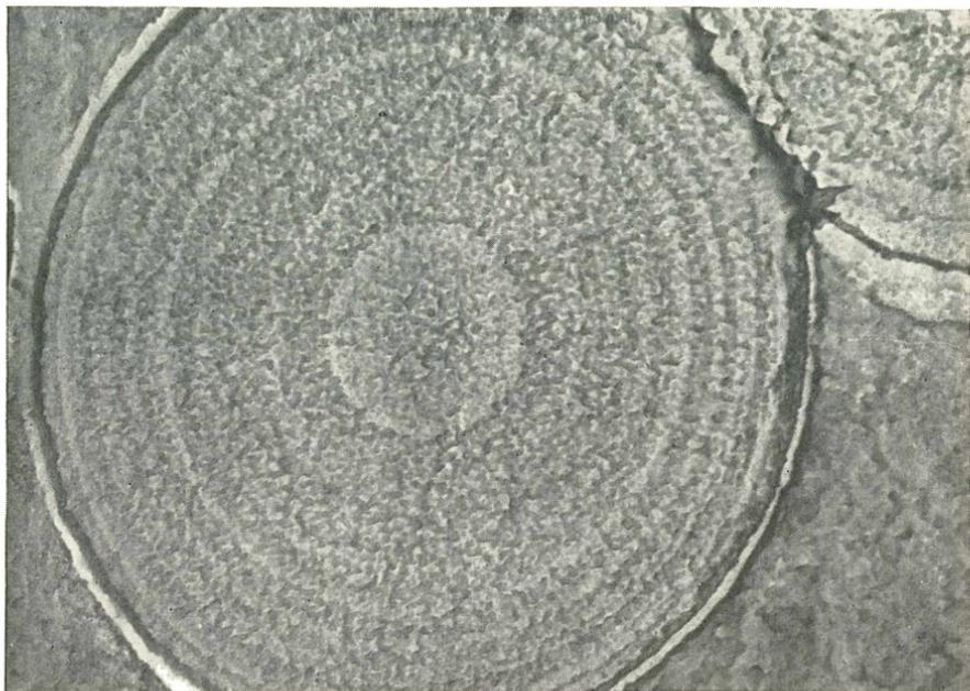
*Fig. 17 Particles of carbonyl iron powder. 15.000:1.*
