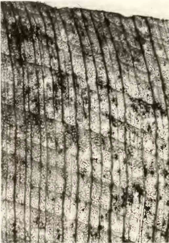
Fig. 8. Cross section (Pfaffing). Wood diffuse porous with 12 growth boundaries and dark rays. \times 15 .
