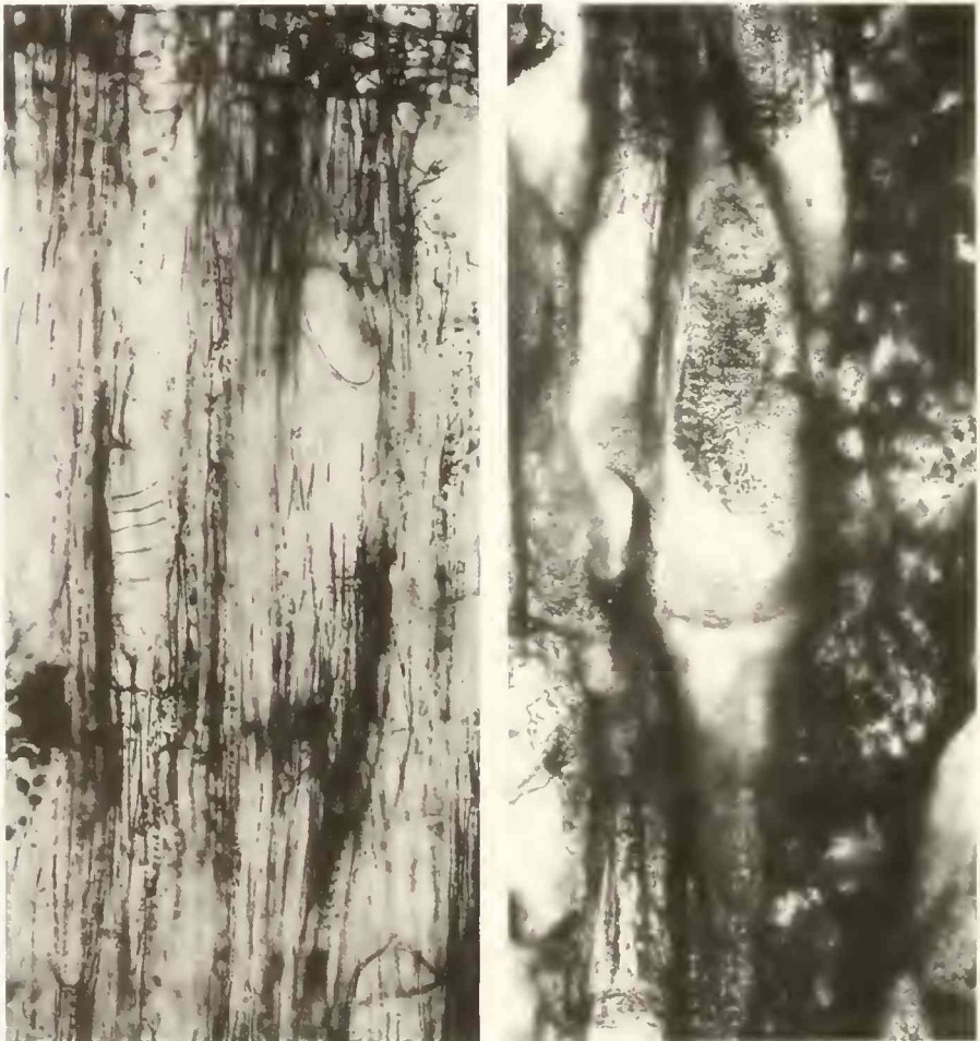
Fig. 15. Radial section (Unterbachham). Left: Vessel perforations simple and scalariform with some bars. Right: Intervessel pits opposite. \times 250 .
