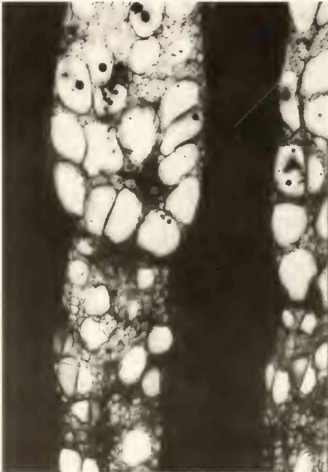
Fig. 11. Cross section (Unterbachham). Growth ring boundary between the dark rays, rays markedly broader on the growth ring boundary. \times 125 .
