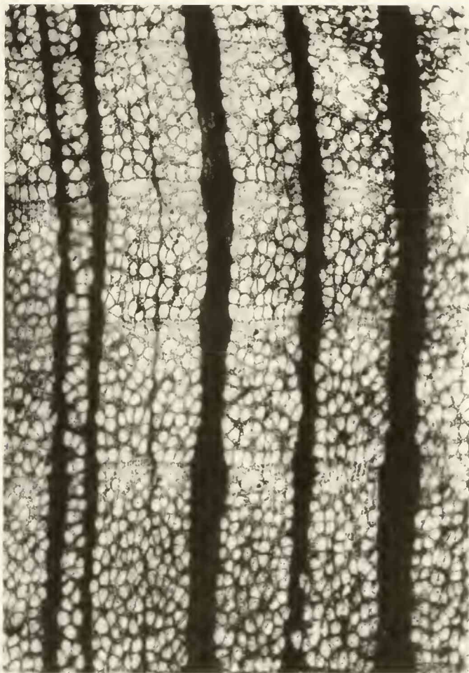
Fig. 1. Cross section (Frankenmarkt). Wood diffuse-porous with five growth boundaries, vessels very numerous, evenly distributed. \times 25 .
