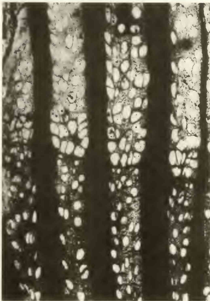
Fig. 10. Cross section (Unterbachham). Growth ring boundary distinct, vessels in the early wood are larger than those in the latewood of the previous growth ring. \times 50 .
