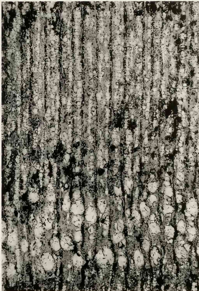
Fig. 1. Cross section. Ring porous wood with marked differences in vessel diameter between late wood and early wood. x 40.
