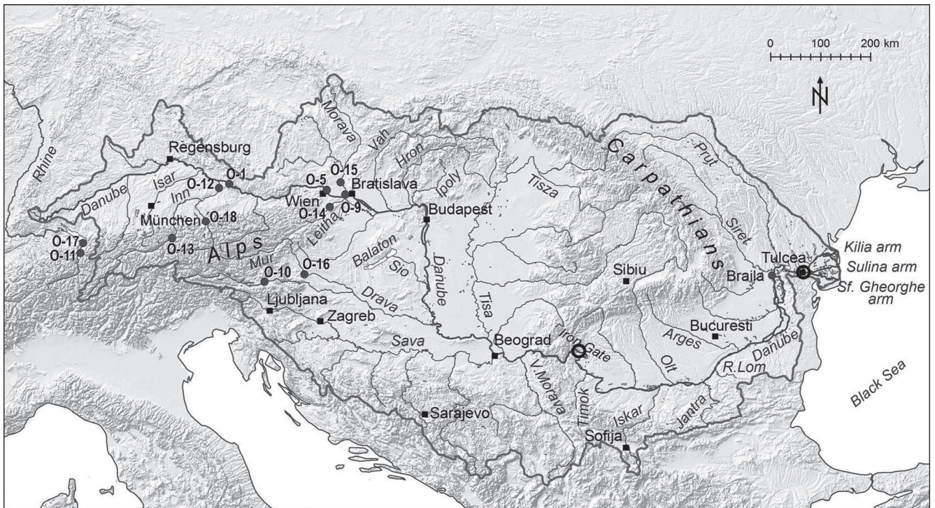
Figure 28: The Danube Basin river system with indication of the proposed sampling points at the Iron Gate and Tulcea as well as the sampling points of the Austrian network for isotopes in river water (Table 4), where long-term isotope records are available (based on ESRI ArcGIS 9.3).
