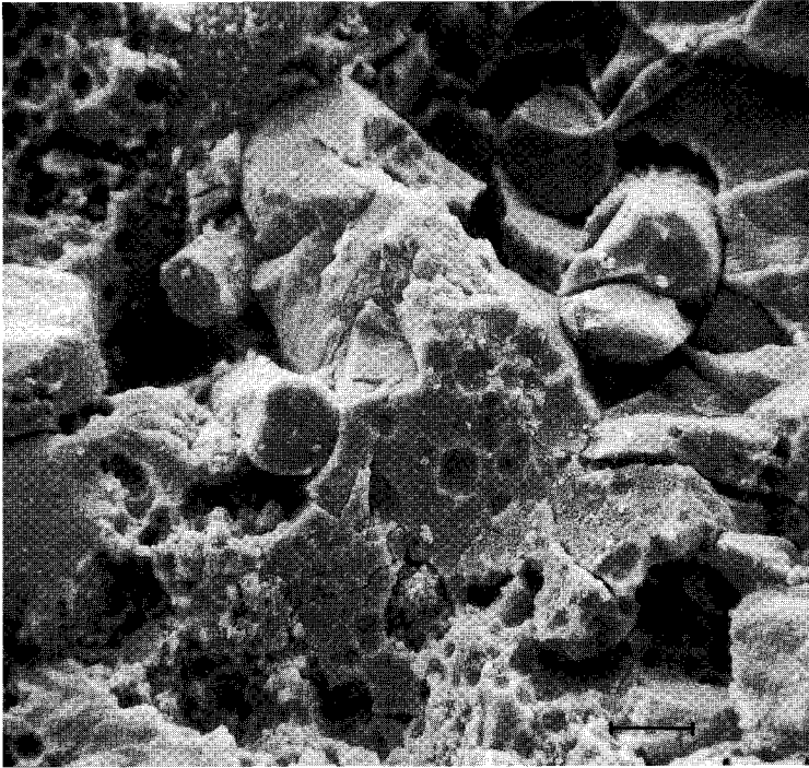
Fig. 36. SEM-Photograph of porous chert; Höf- lein Formation. Höflein 8, 2843.2 m. Length of scale = 36 \mu .
