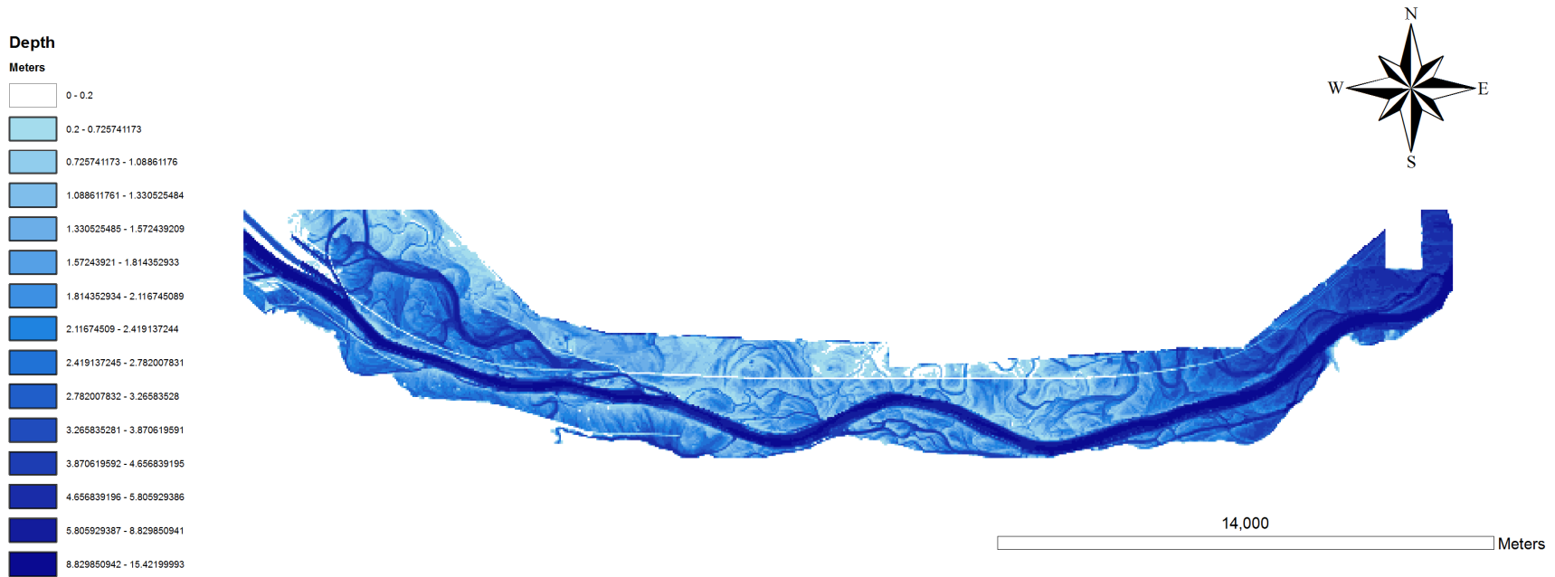
Figure 17. Flood simulation results for the future scenario. Where (a) is 100-year flood event maximum flow depths, (b) 30-year flood event maximum flow depths, (c) annual flood event maximum flow depths.
