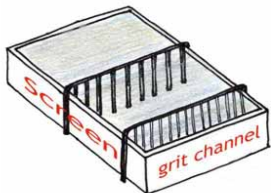
fig. 110: screen and grit channel
