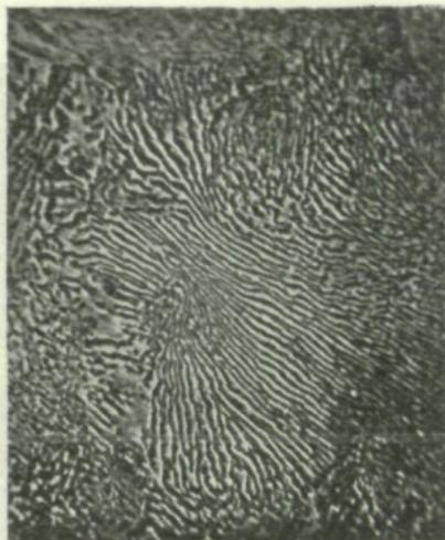
Fig. 5. Stahl ( $0.9\%$  C),  $V=1000$  (Perlit).
