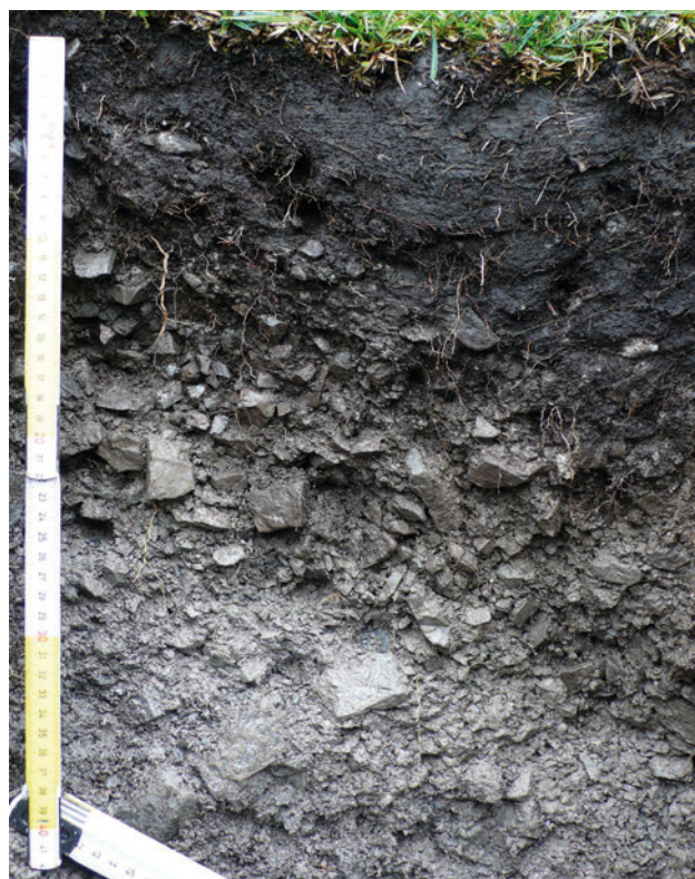
Fig. 3: Soil profile 1 from dolomite debris in Brixenbach valley (1 000 m): the multiple layers of the parent material are clearly identifiable from the varying skeleton content. Photograph by C. Geitner 2008.
