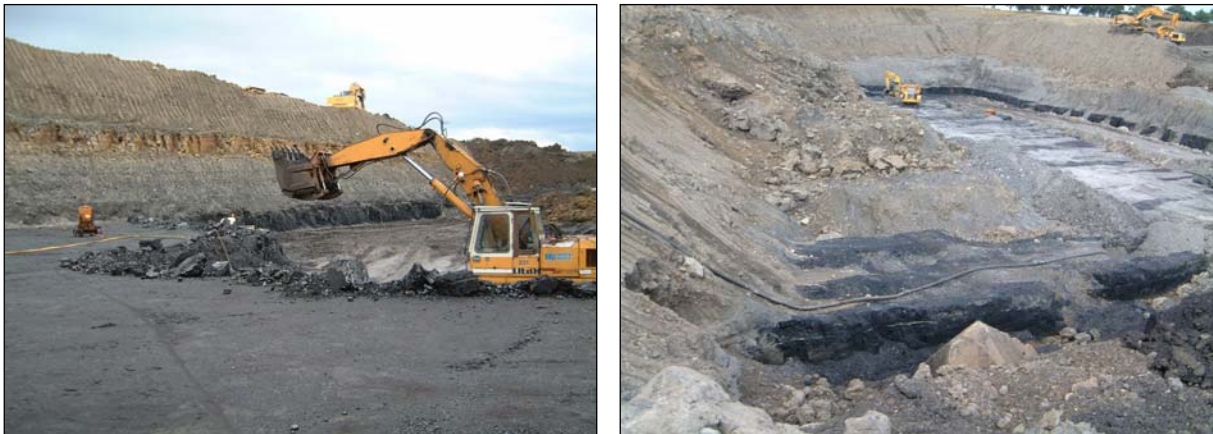
Fig. 2: Opencast coal mining operations: (left) working bench in front of the highwall of a shallow pit. (right) advancing loose-wall (on left) behind working bench
