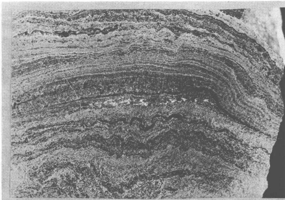
Fig. 3: Excellent finely folded layered structures of magmatite and hematite in amphibolite schist. – Fischerzeche near Přísečnice/CSSR (Pressnitz series). Scale 1 : 1 (from WEINHOLD 1977).
