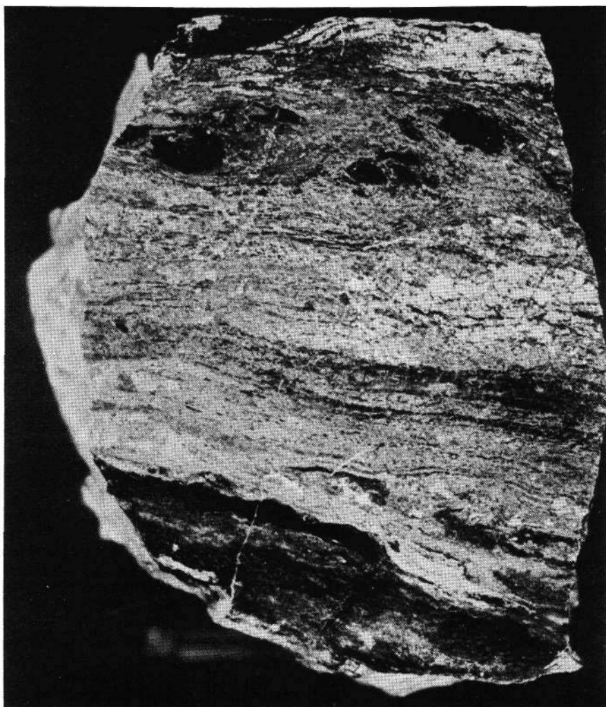
Fig. 2: Layered compact ore consisting of pyrite (white), melnikovite and marcasite (light grey), rhythmically alternating with cassiterite (dark grey) as well as quartz-chlorite schist (black; partly with boudinage formations). The layered structure points to light folding. – “Felsite horizon” of Halsbrücke (Pressnitz series), ore horizon II, 350 m level, scale 1 : (from WEINHOLD 1977).
