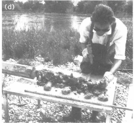
Plate 5.3.1. Significant steps of the sampling procedure: (a) Liquid N_2 is poured from a five kg Dewar vessel into the corer, which is protected by a wooden mantle. In the left hand of the operator is the distributor (Fig. 5.3.1). (b) The core is extruded with the help of a lever. (c) The frozen core. (d) The core is segmented.
