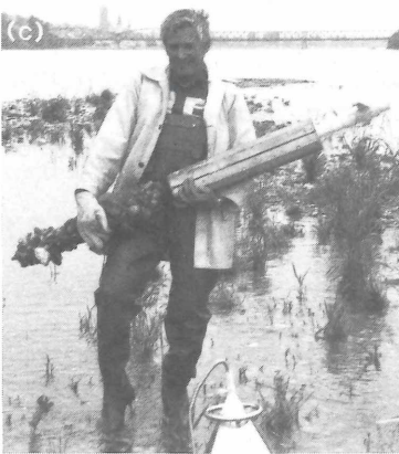
Plate 5.3.1. Significant steps of the sampling procedure: (a) Liquid N_2 is poured from a five kg Dewar vessel into the corer, which is protected by a wooden mantle. In the left hand of the operator is the distributor (Fig. 5.3.1). (b) The core is extruded with the help of a lever. (c) The frozen core. (d) The core is segmented.
