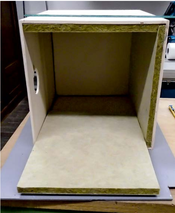
Fig. 2. Attaching the insulation boards, photo: Beate Maria Pomberger.
