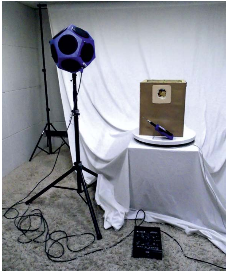
Fig. 8. Measurements of the effectiveness of the sound-reduced chamber, photo: Beate Maria Pomberger.
