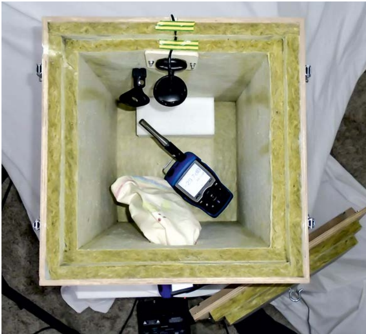
Fig. 7. Measurements of the effectiveness of the sound-reduced chamber, photo: Beate Maria Pomberger.
