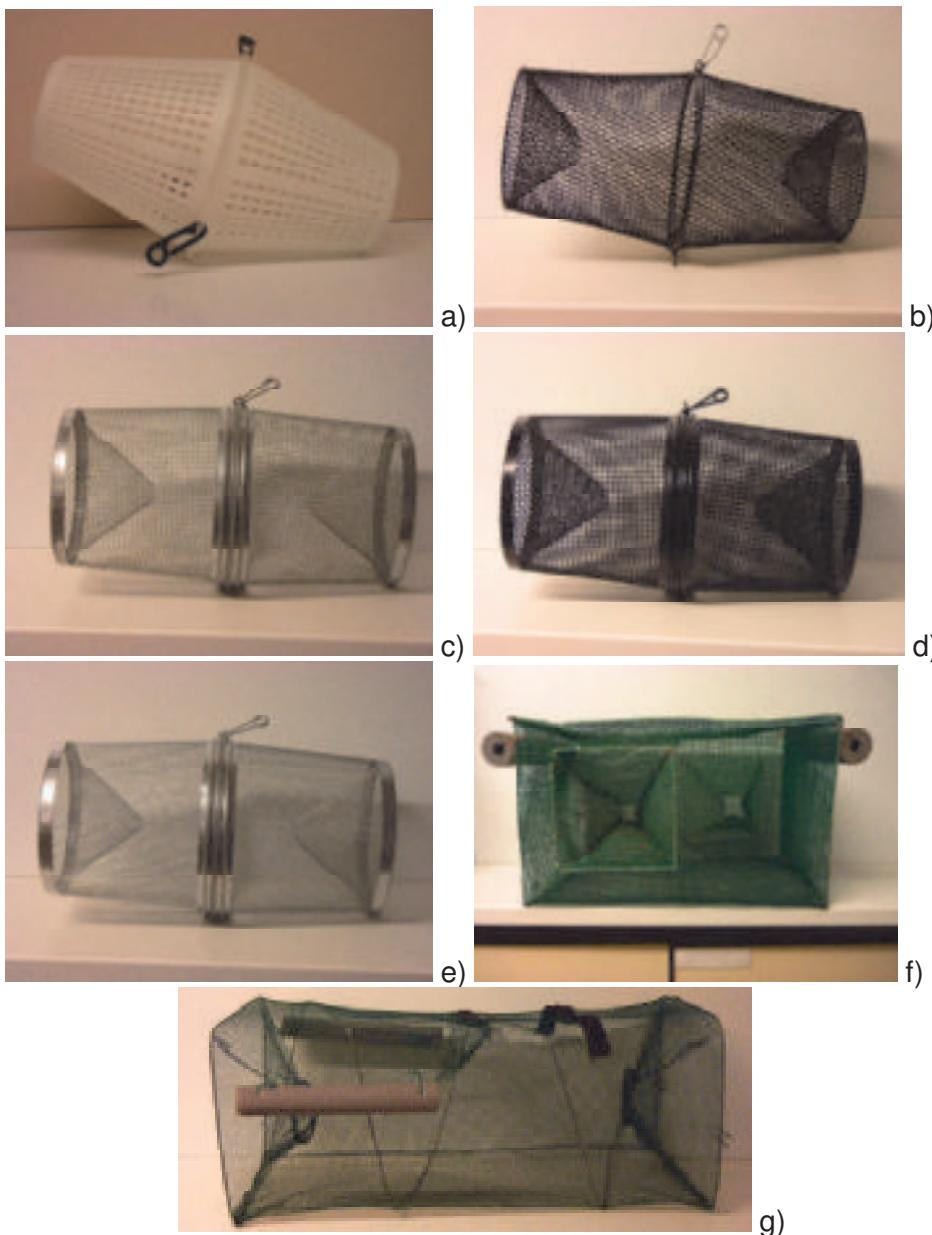
Figure 1: The seven types of funnel traps tested: (a) Minnow trap plastic, (b) Minnow trap "Cuba", (c) Minnow trap "Gee 40", (d) Minnow trap "Gee 40 optimized", (e) Minnow trap "Gee 48", (f) HENF trap (model I, a modified model II HENF-LAAR is now available ), (g) Collapsible nylon trap. Photos: A. Kronshage.
