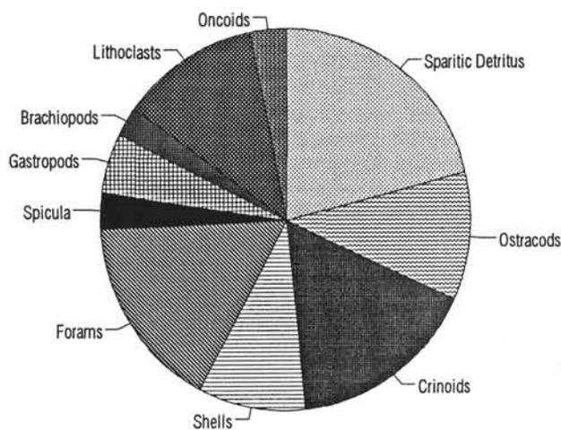
Text-Fig. 18. Composition of the sponge layer in Quarry XXXI as determined by point counting of two thin sections (864 counts; MF 2.2, chapter 2.4.2.1). Micritic and microsparitic matrix making up 40% of the counts is not shown. "Shells" are recrystallized bioclasts, most likely of broken bivalves and ammonites. The microfacies is dominated by crinoids and foraminifers.
