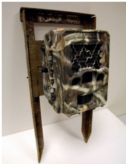
Fig. 2 Camera fixed on the platform is ready to be installed into the beaver burrow. Photo by A. Ulevičius.
