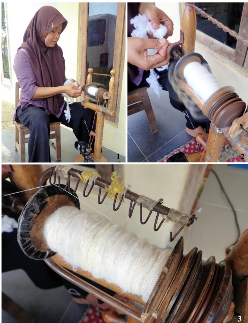
Figs. 1-3. Indonesia, Yogyakarta. Eri-silk ( Samia ricini ) is hand-spun. The spinning wheel is driven by a small electric motor.
