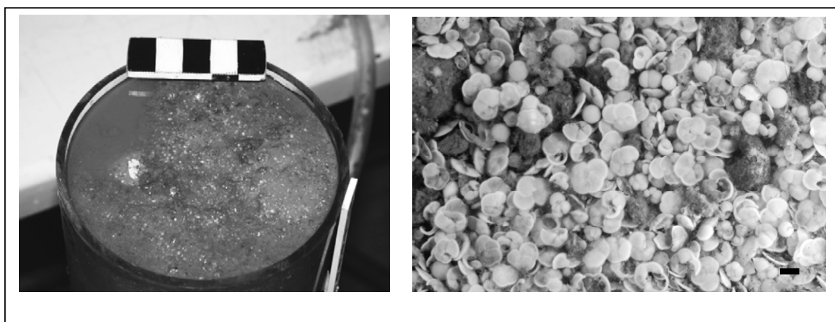
Fig. B: Globigerina ooze from the Guinea basin sampled at 5100 m water depth and sieved residue of the sediment (right picture). scale bar left picture: 50 mm, right picture: 1 mm.
