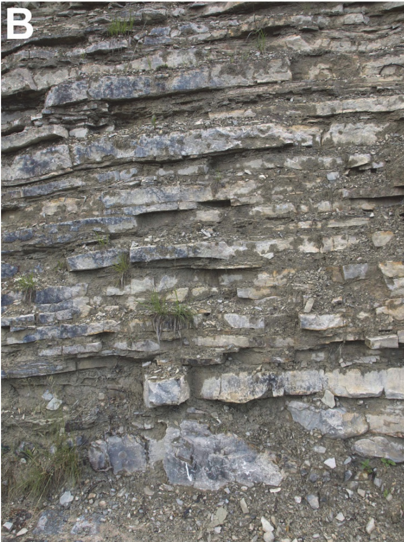
Fig. 12: Road cut with the Oberalm Formation along the road to Krispl. A) Outcrop situation before the fixation of metal nets. B) Dm-bedded limestone beds with intercalated green marls.
