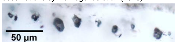
Fig. 3. Coexisting liquid-rich and vapor-rich inclusions in an FIA from the shallow, high-gradation part of the system (100 m present day depth).
