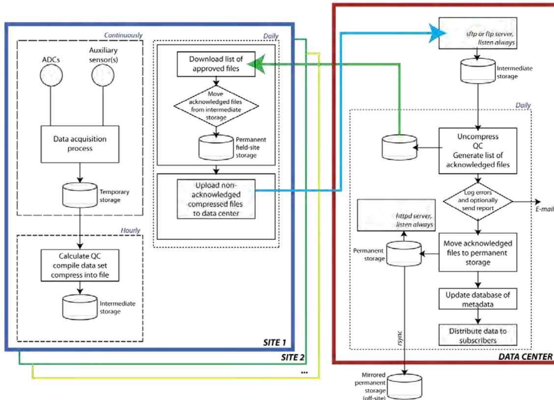
Fig. 4: Overview of data transfer system principles.
