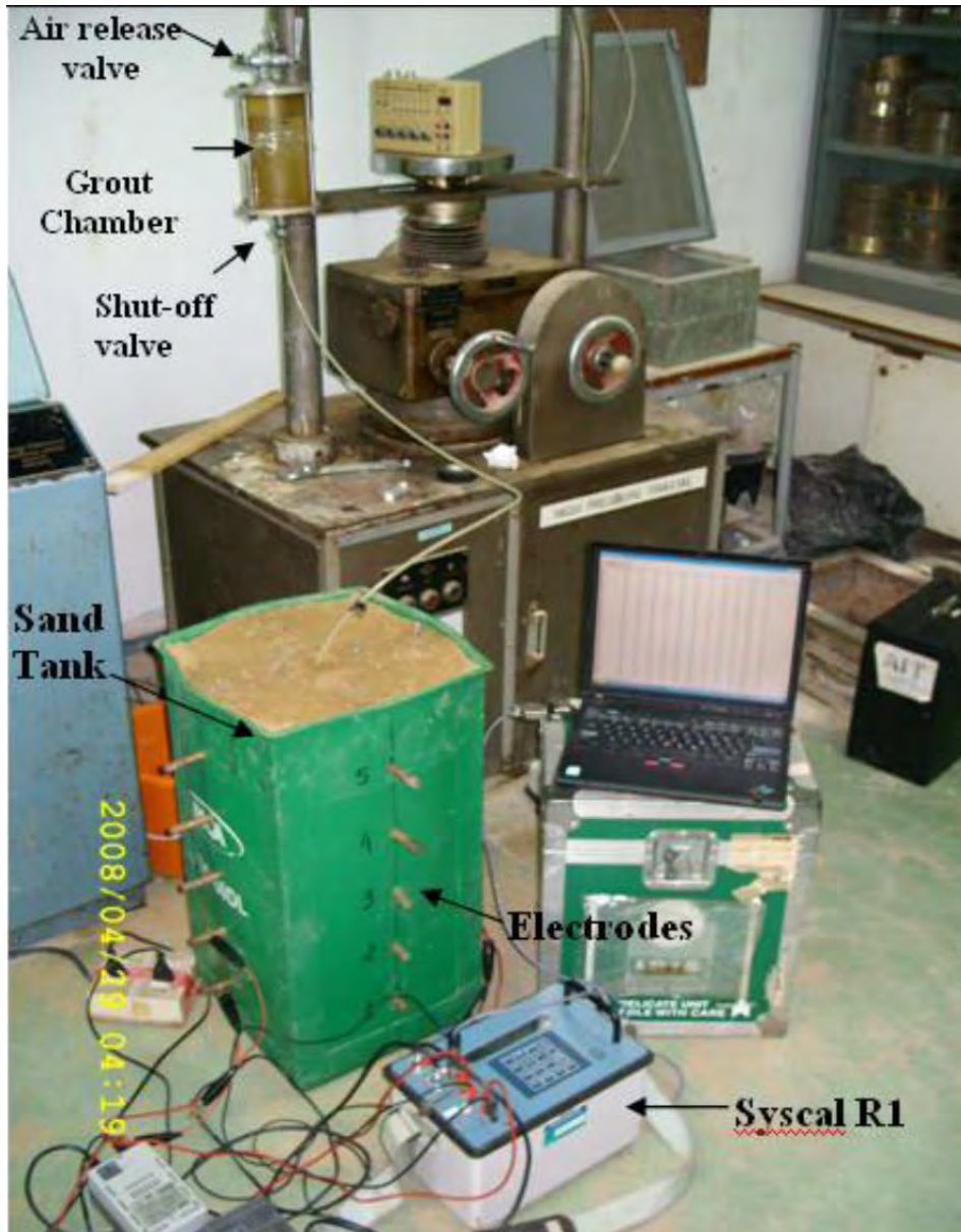
Fig. 12: View of the grouting and ERT setup.
