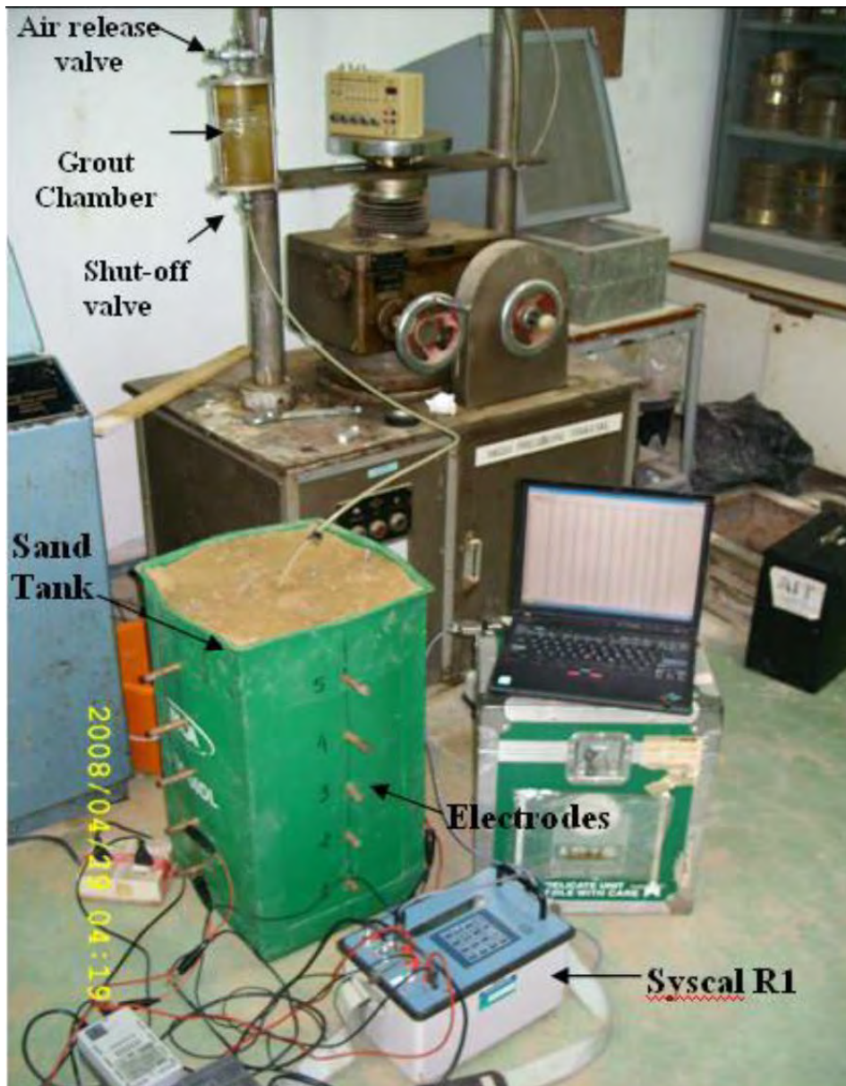
Fig. 12: View of the grouting and ERT setup.
