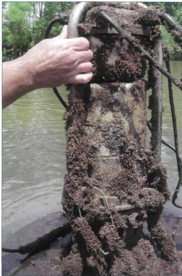
Fig. 4: Bryozoans ( Plumatella rugosa ) growing on a submersible pump for a decorative fountain in a pond in Centerville, Ohio, USA.
