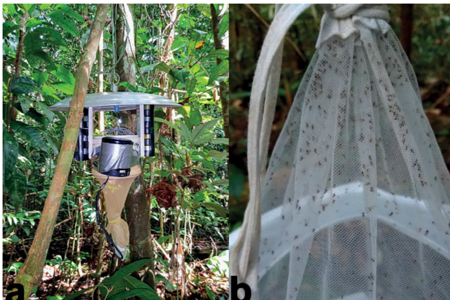
Fig. 2. Method of Corethrella collection. a. CDC light trap with a speaker attached playing looping of frog species songs from the ‘sapoteca’ frog library ( https://ppbio.inpa.gov.br/sapoteca/paginainicial ). b. Cage with dozens of Corethrella collected.
