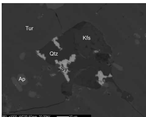
Fig. 12. Quartz (Qtz), K-feldspar (Kfs), tourmaline (Tur), apatite (Ap) and small grains of synchysite (Sy).
