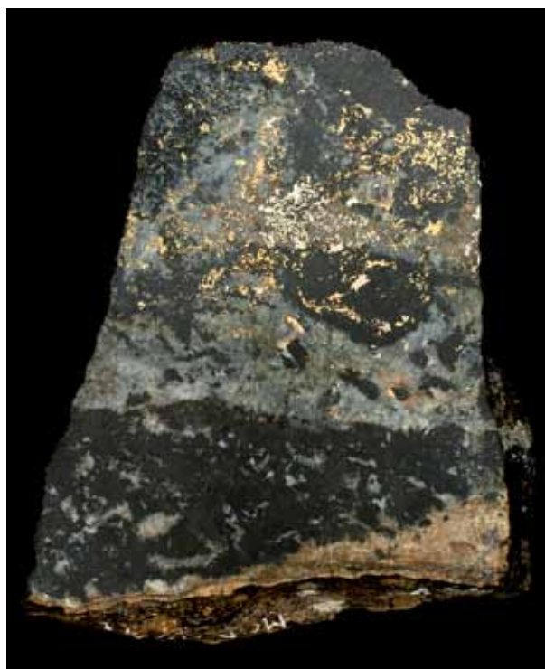
Fig. 5. Banded mineralization of chalcopyrite and pyrite in tourmaline (black) and quartz. Vecchia Bedovina-M. Mulât mine. The maximum length of the sample is 8cm.
