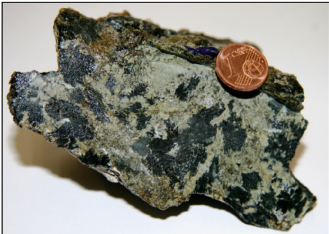
Fig. 10: Hand specimen of the Gufidaun metagabbro showing cm-size black amphibole crystals.
