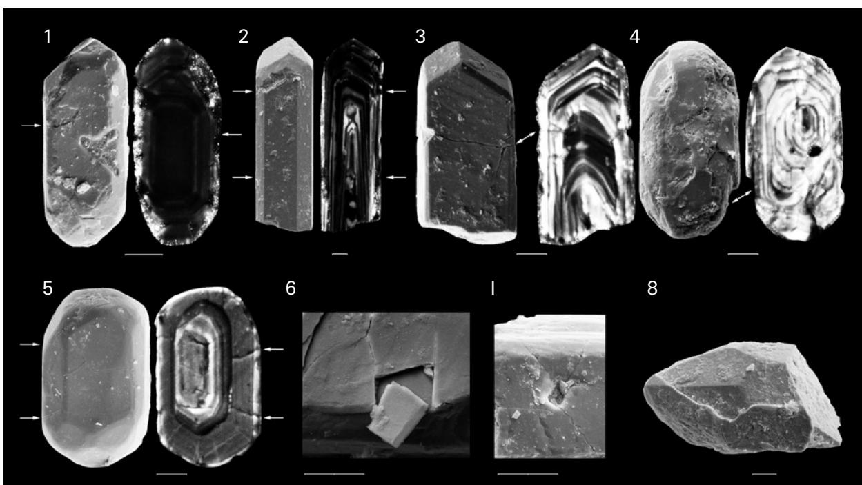
**Fig. 5.** The two different types of cracks in zircons: **1** and **2** are caused by collision during transport, **3** results from collision and from volume extension, **4** and **5** are caused by volume extension, **6** shows delamination of layers, **7** are cracks induced by collision, **8** is a zircon grain with partly removed outermost layer (scale bar: 20 µm).
