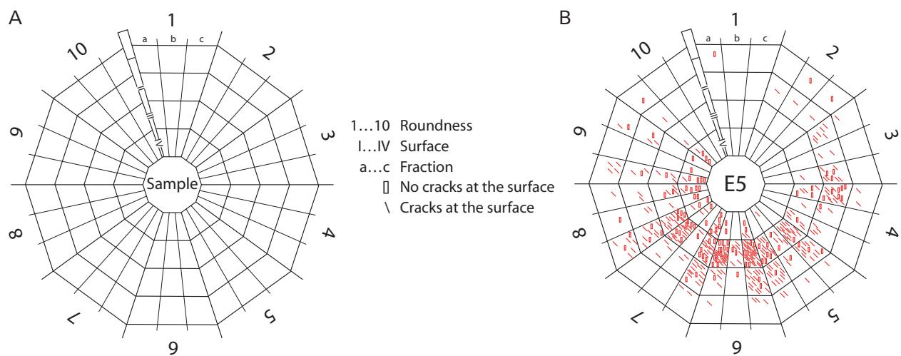
**Fig. 8.** Spider plot showing the interrelations between roundness, collision marks, type of fraction, cracks at the crystal surface, and location for sample E5 (Elbe River in Groß Schönebeck).
