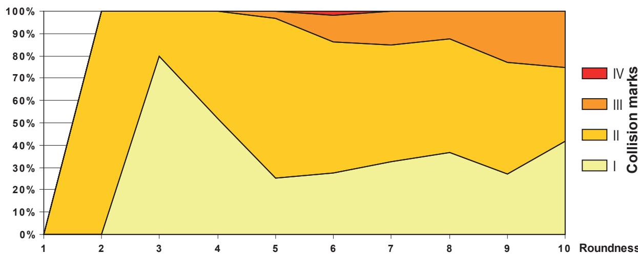
**Fig. 7.** Diagram illustrating the interrelation between roundness and collision marks for sample NAM-O-23 (Cunene River near Ruacaná, Namibia).
