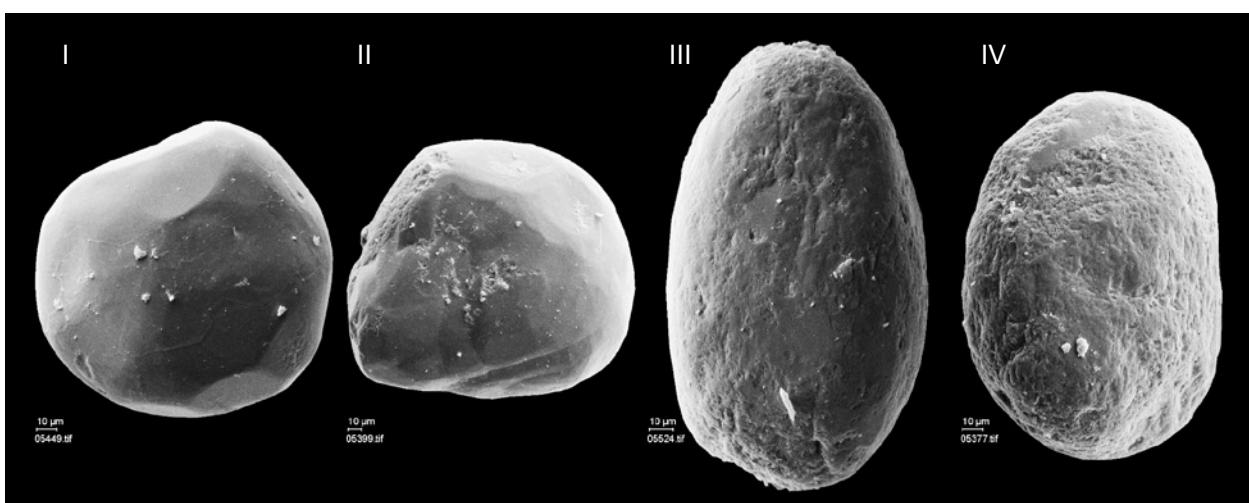
**Fig. 6.** Typical zircon grains of the four classes of collision marks (**I** to **IV**, scale bar: 10 µm).
