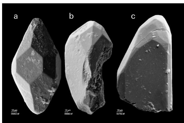
**Fig.** 3. Typical zircon grains representing the three classes of fracturing (a to c, scale bar: 10 µm).
