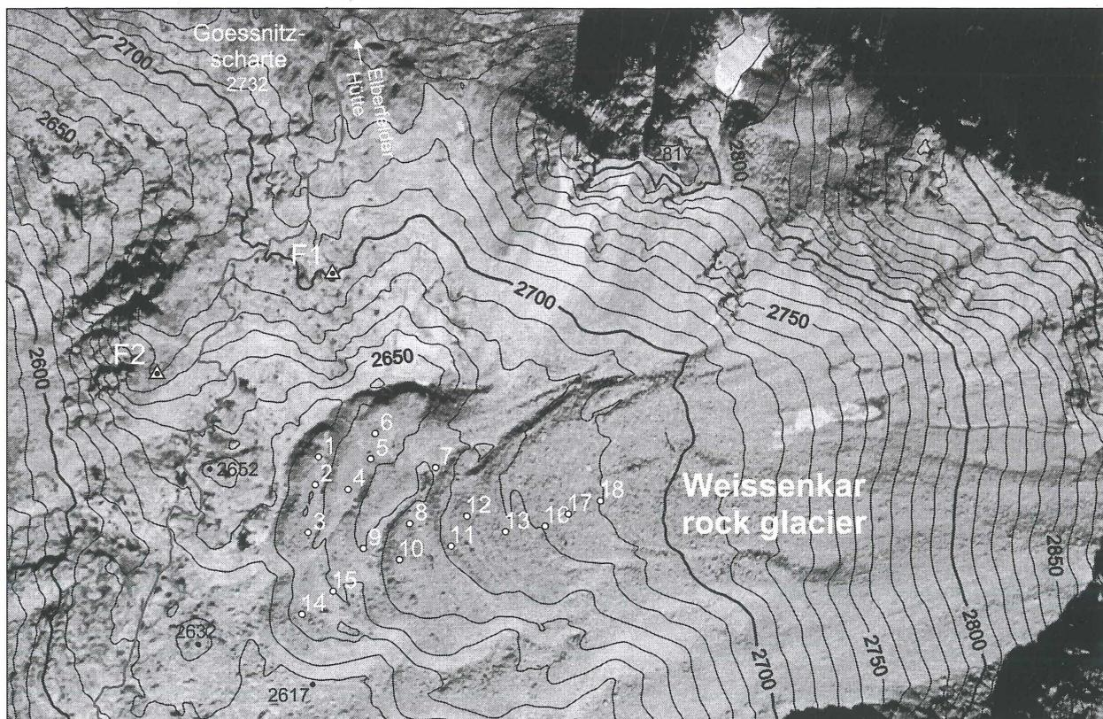
**Figure 3:** Orthophoto map showing Weissenkar rock glacier. F1 and F2 are geodetic reference points. Points 1-18 are object points fixed by brass bolts on large boulders of the rock glacier surface. The color photograph was taken on 18 September 2002 by the Austrian Federal Office of Metrology and Surveying. Photograph © Amt der Tiroler Landesregierung, 2004. Contour lines derived by (manual) photogrammetric mapping.
