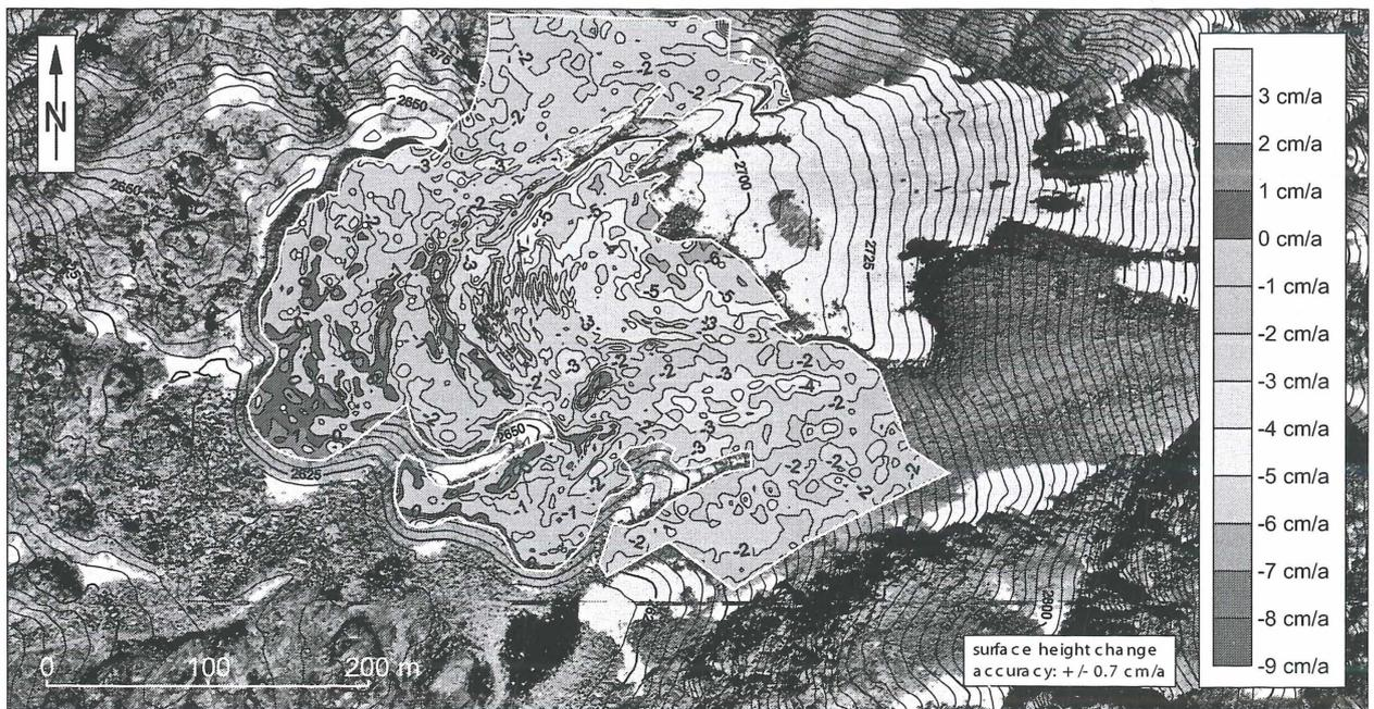
Figure 8: Mean annual surface height change (cm a<sup>-1</sup>) for the time interval 1974-1998. Surface height change has been derived from 3D displacement vectors and surface slope data assuming surface parallel flow of particles.
