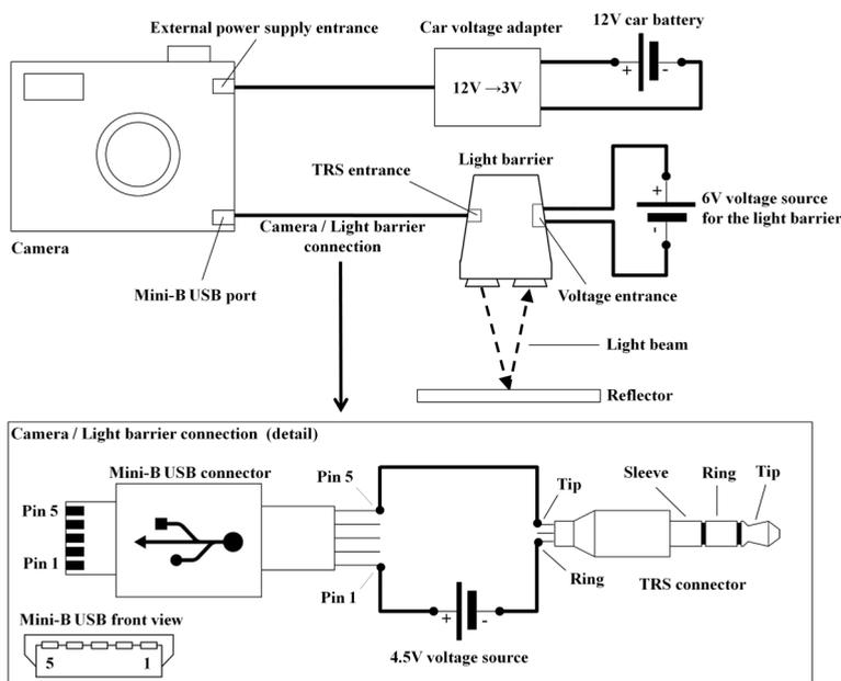
Fig. 1: Wiring scheme of the camera trap assembled by the first author.
