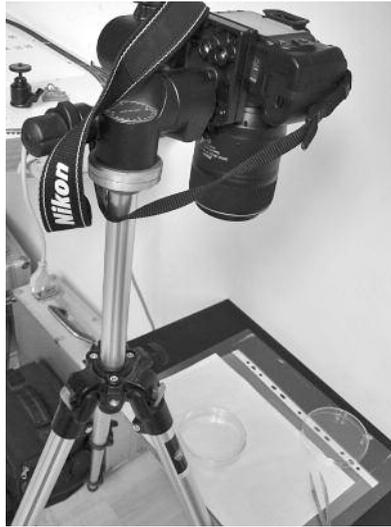
Fig. 3: Camera set-up for photodocumentation including DSLR camera (Nikon D3000), lens (AF-S Micro Nikkor 105 mm), flash unit (not shown) and tripod with tripod head (Manfrotto 410).
