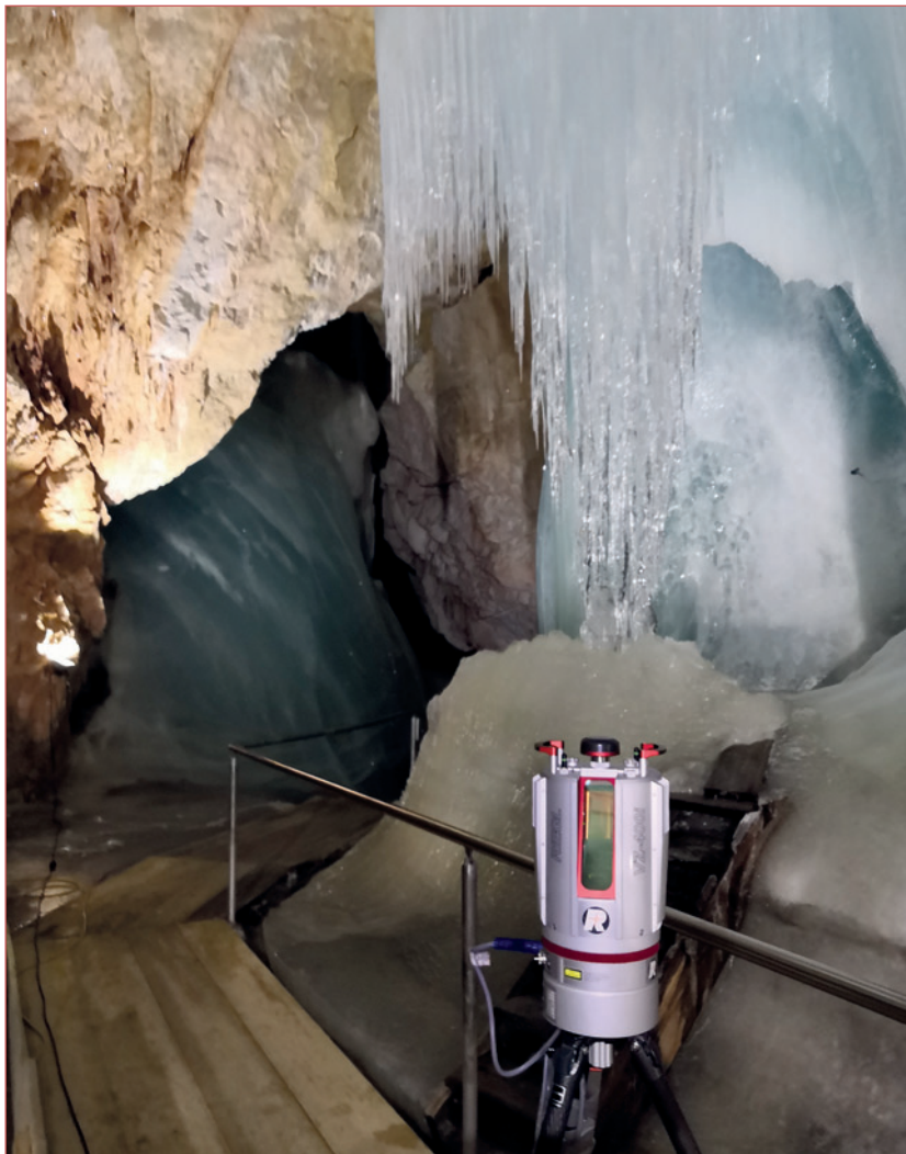
Fig. 1: The RIEGL VZ-400i terrestrial laser-scanner mounted on a tripod on the visitor walkway of the Eisriesenwelt.
