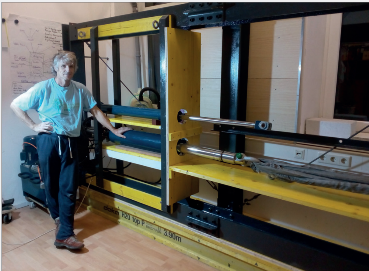
Abb. 2: Zerreißmaschine. Fig. 2: Experimental setup.
