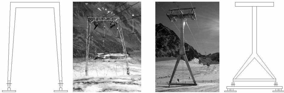
Figure 4: Possible support structures: Portal frame for surface lift (left) and Y-shaped pillar for aerial lift (right).
