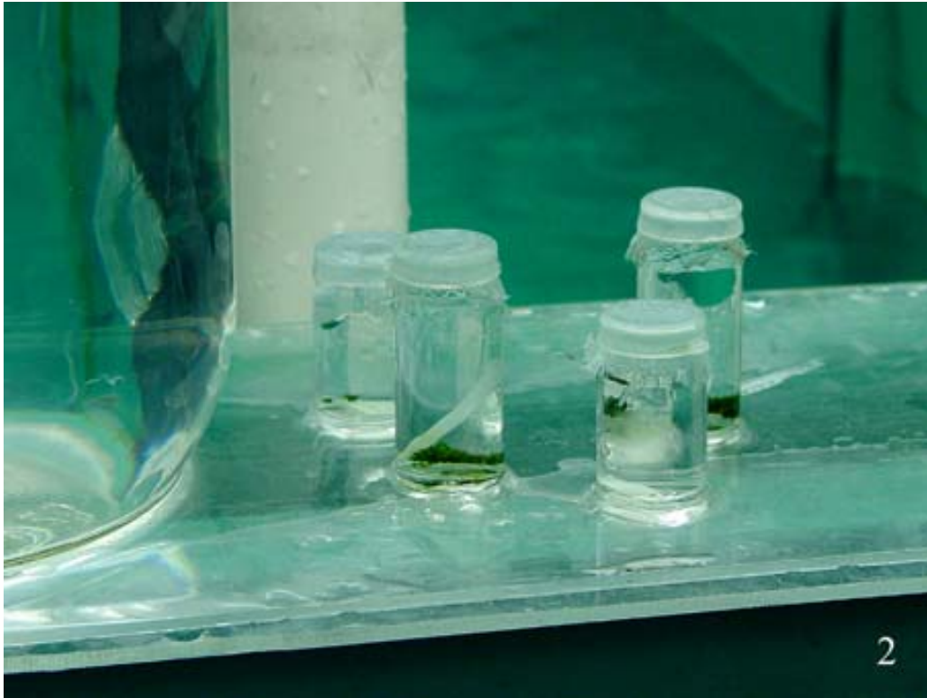
Fig. 2. Egg incubation containers with Nitex® mesh held over openings with modified lids. Living Stream in background.
