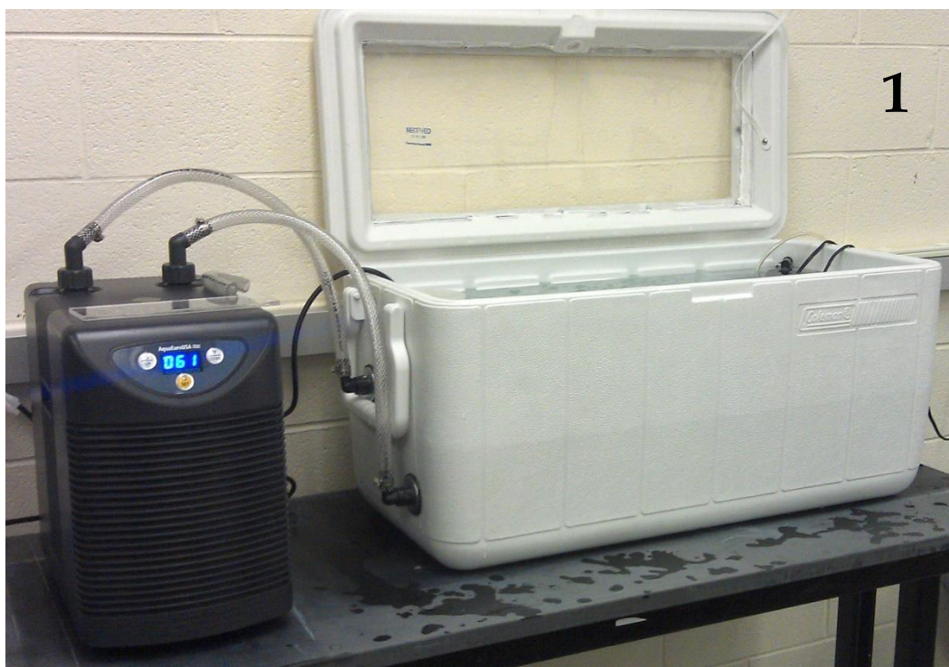
Fig. 1. Artificial stream used in rearing immature aquatic insects in the laboratory.
