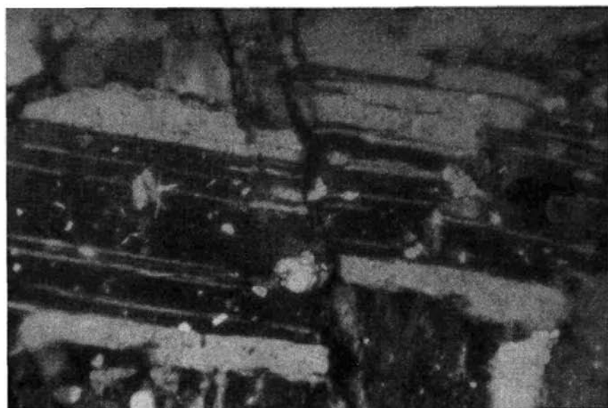
Fig. 10. Flaser granite. Microfault dislocating an albite crystal. The plane of the microfault strikes E-W. (Wilhelmshof, NO).
