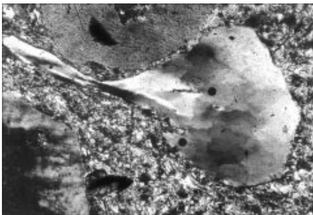
Text-Fig. 39. Splinters of deformed quartz crystal in felsitic granite porphyry. d.p. LT 363; 1.5 km W of Rottal. Magnification \times 40 ; crossed polars.
