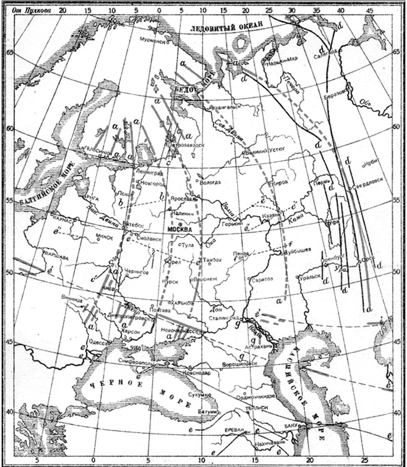
Text-Fig. 11. KARPINSKY'S (1887) map of structural trend of the Russian craton and its surroundings. Thick dash lines – trends of Precambrian rocks. Note their continuity beneath the platformal cover. Thick solid lines – Uralian trends. Thin solid and dash lines – Mesozoic trends that were called KARPINSKY lines by SUESS.
