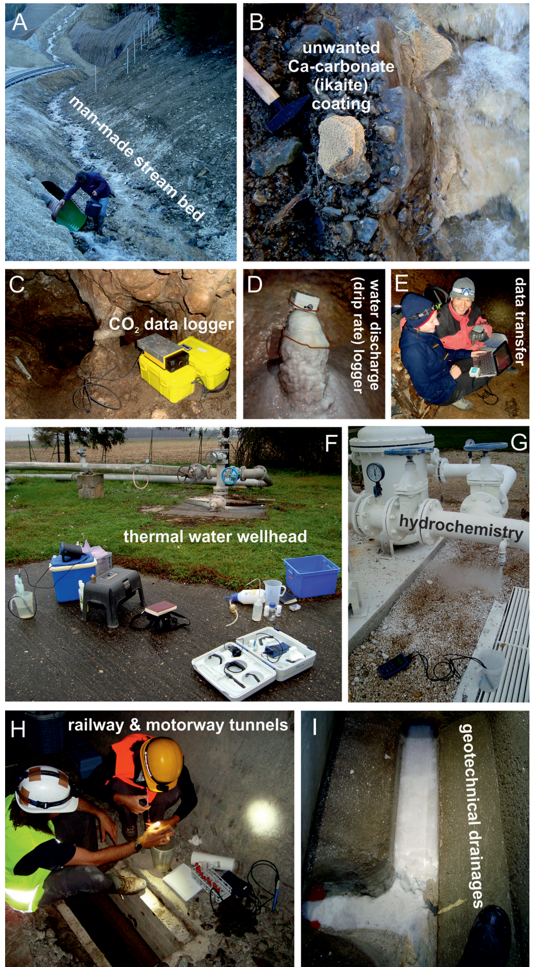
Text-Fig. 7. Impressions from natural and geotechnical settings of environmental monitoring. A, B) Regular monthly monitoring and process understanding of unwanted Ca-carbonate precipitation and associated hydrochemical alteration in a human-made stream bed. C, D, E) Multi-annual bi-monthly (cave visits) and continuous (data loggers) cave monitoring including cave air, seepage waters and solid precipitates (speleothems) in different cave chambers. F, G) Observation of fluid-solid interaction targeting scaling and corrosion processes impairing deep wells for geothermal energy production. H, I) Monitoring of site-specific mineral precipitates clogging drainages in different tunnels.
