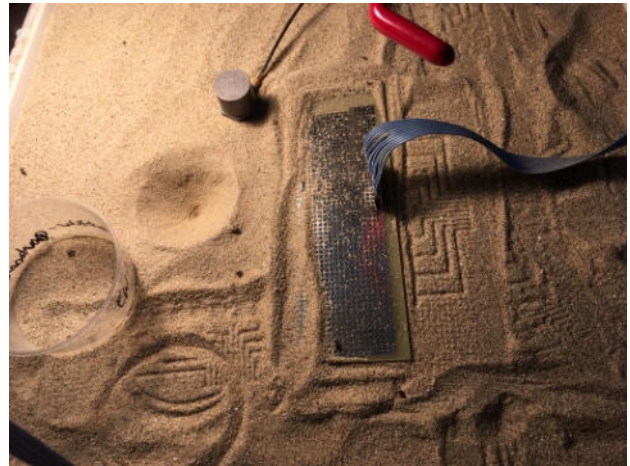
The board with attached piezo-transducers (under side) was used to transmit signals to the sand surface.
